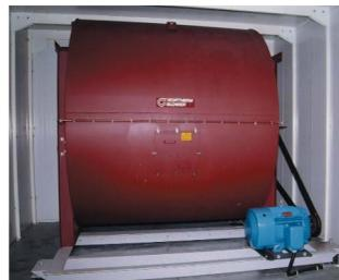
A 75-hp motor and 75,000 cfm blower creates wind speeds of up to 160 km-h.
