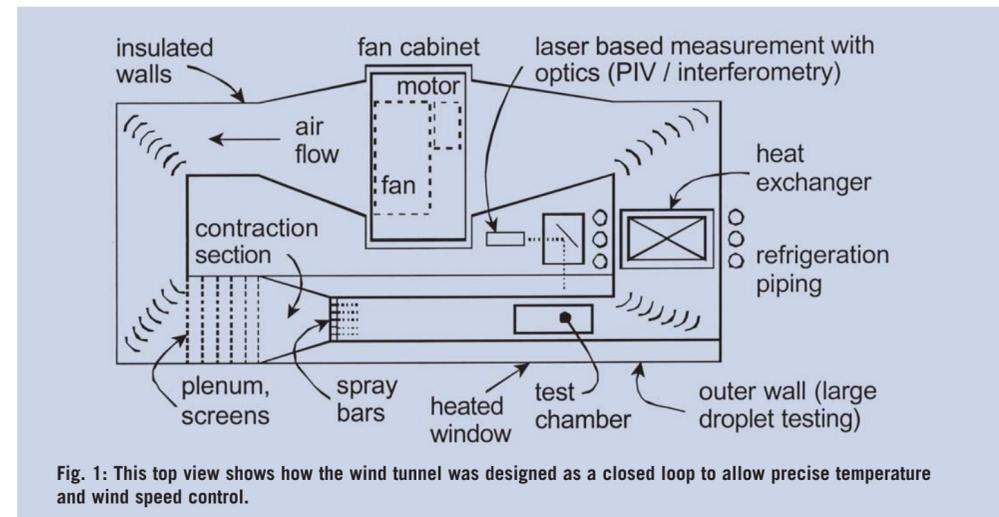
Fig. 1: This top view shows how the wind tunnel was designed as a closed loop to allow precise temperature and wind speed control.
